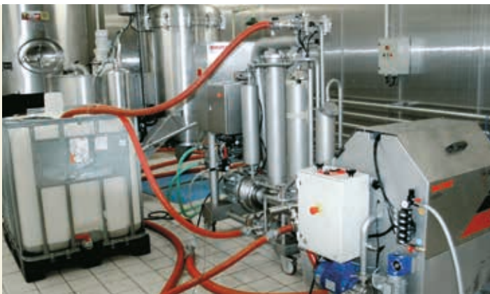
Juice lees filtration installation
